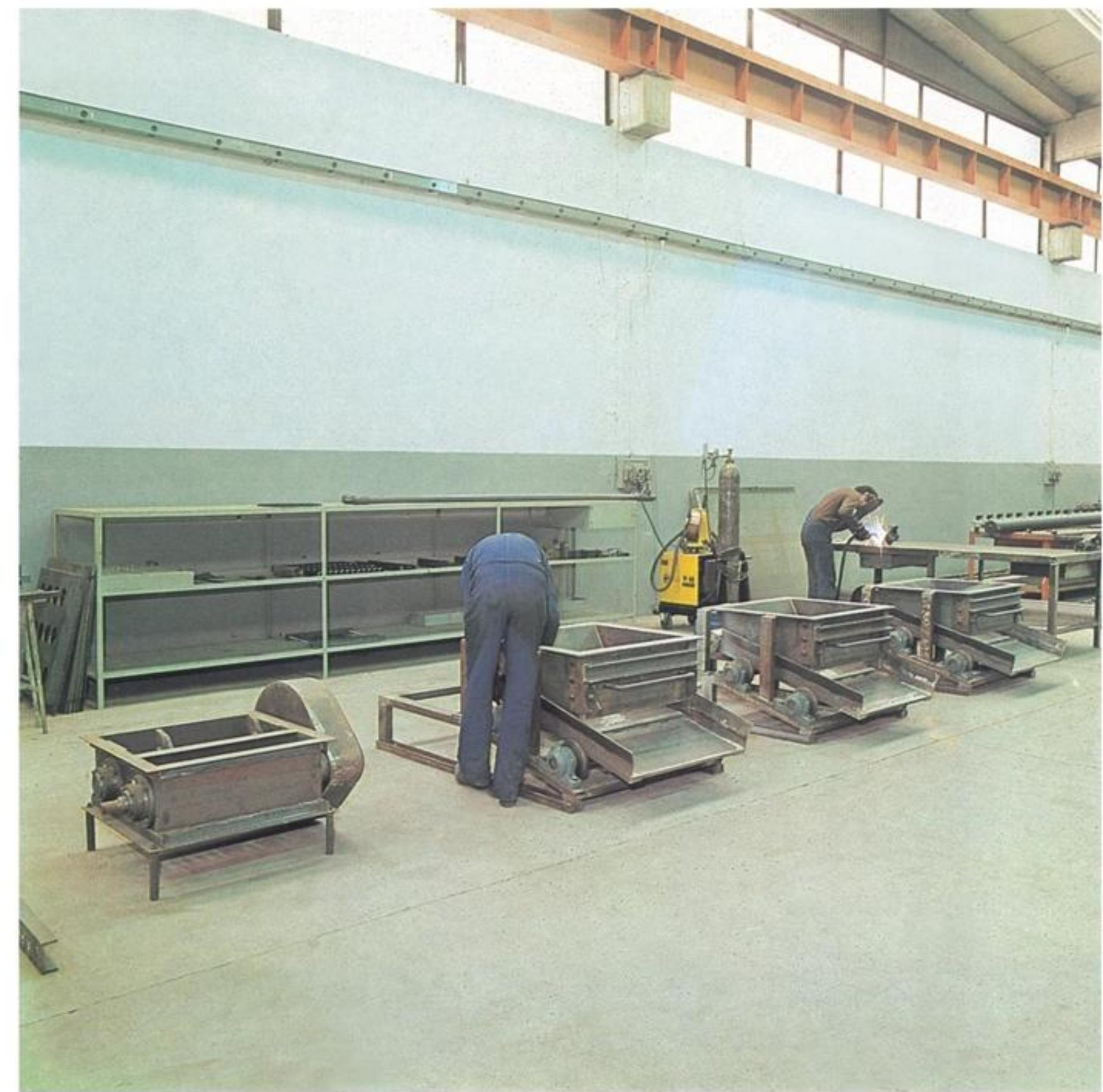
In this department, machines for the internal transportation of granulated or powdered products are manufactured in a wide range of models:
